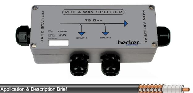
The Becker UHF 4-Way Splitter is used to split the main arterial line into three separate Leaky Feeder Arterials. In doing so the RF power is divided equally between the four resultant arterials. The DC Power may also be routed in various directions by opening and closing the on board jumpers. DC injection screw terminals also allow this unit to be used as a make shift "Power Coupler". Additional jumpers allow the technician to internally terminate the unused RF ports.
