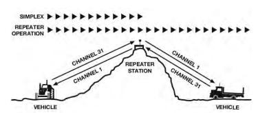
Your XRS-370C radio allows you to enable or disable Duplex mode on individual repeater channels. In this way any repeater channels that are not being used with repeaters in your area can be used in Simplex mode for normal direct radio-to-radio communications.
